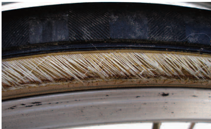
The sun cooked this sidewall in about three months of summer storage. This particular sidewall is especially tough, and has layers underneath still intact. But still; time to go.
