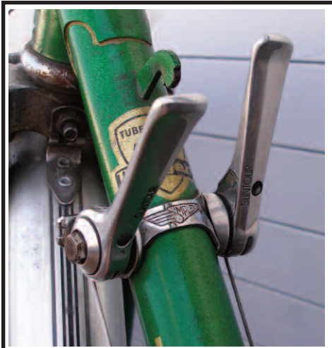
Problem: His plastic Simplex down tube shifters broke, and his bars (on this old, low-end Peugeot) didn't have enough room for thumb shifters, and wouldn't accept bar-end shifters.
