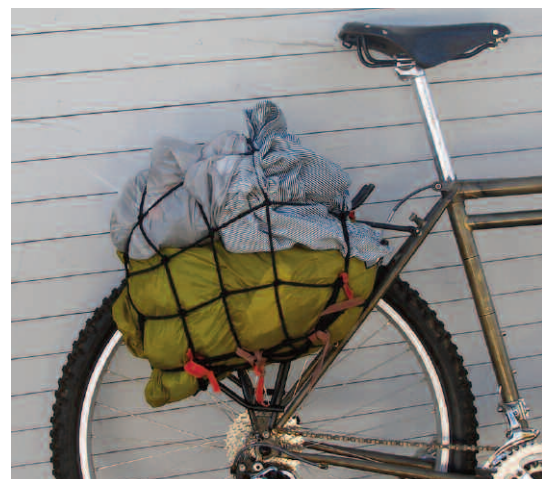
Using the hooks, the Nanners contain the load and hold it to the rack. Loading is a cinch. It looks like heck, but it works great. You'll figure it out.
