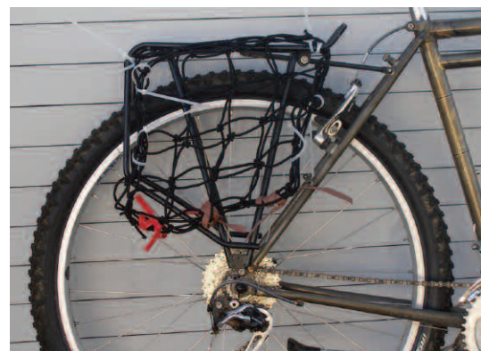
Shown here empty and with zip ties holding the sides closed. It's better to use the hooks. Easier to load.
