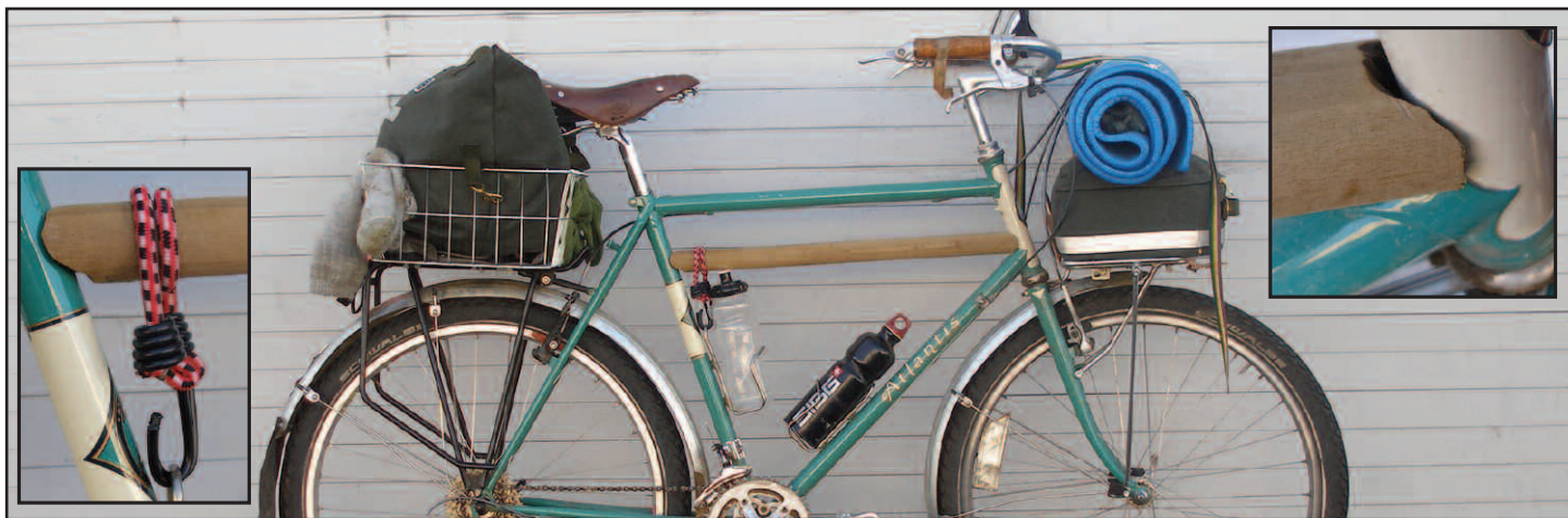
Top left and right show precise hand-miters. Bottom left photo shows ingenious way to keep the rod from slipping. Bike as shown after a successful Sub-24-Hour overnight in the local hills
