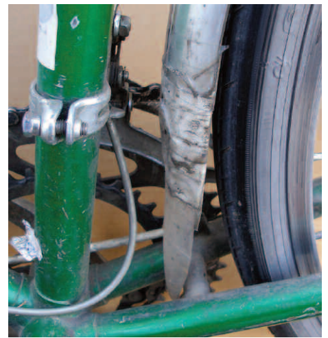
Problem: He "shifted" his fender rearward to give more coverage back there, but it left a gap on this other end.
