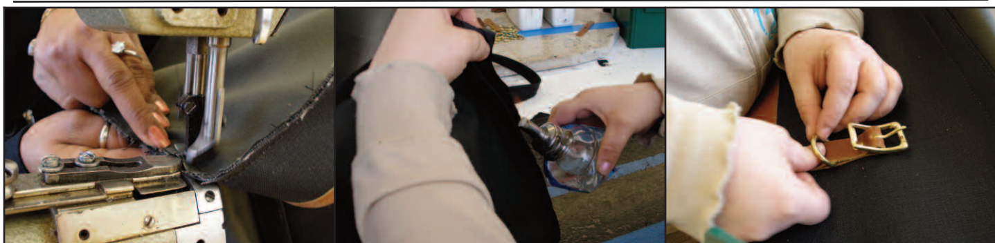
Sewing the bags, melting the thread ends, installing a buckle.
